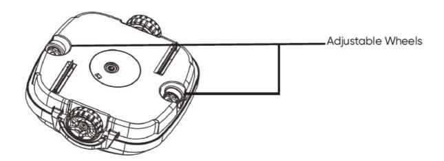
To adjust the wheel, open the lock buckles and remove the top cover. Locate the 2
