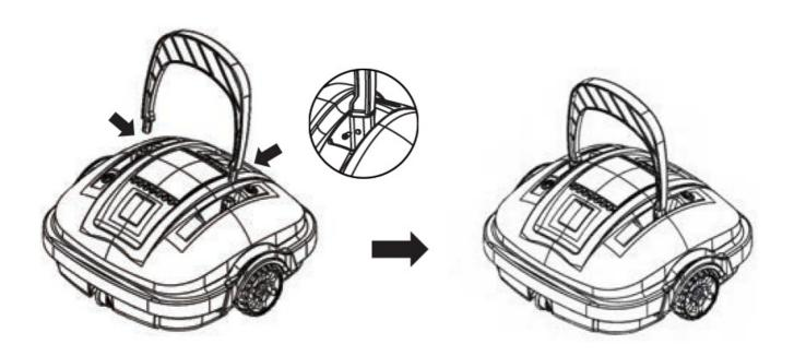
**Note:** The installation direction of 2 screws is opposite.
