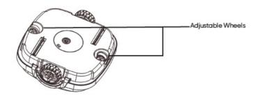
To adjust the wheel, open the lock buckles and remove the top cover. Locate the 2 adjustable wheels. Detach the wheel by pushing the wheel stem catch. Select the correct combination and insert the wheel until the catch clicks.
