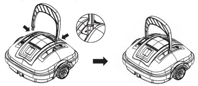
• Install the scrapers to enhance the suction effect if the pool floor is full of debris or particles. It is not recommended to install the scrapers if the pool bottom is uneven or full of pits, which prevents the cleaner from getting stuck on the rough floor.
