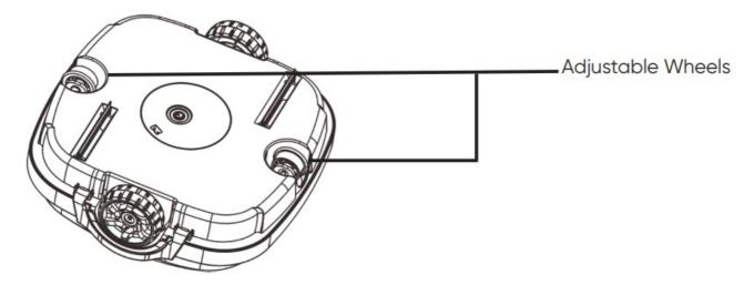
• To adjust the wheel, open the lock buckles and remove the top cover. Locate the 2 adjustable wheels. Detach the wheel by pushing the wheel stem catch. Select the correct combination and insert the wheel until the catch clicks.
