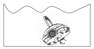
Hold the robotic cleaner in its upright position and slowly release the product. The product shall slowly sink to the pool floor. In case the cleaner is flipped upside down, use the floating handle to correct its orientation.
