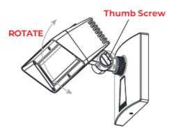
• Loosen the thumb screw and adjust the angle of the fixture. Tighten the thumb screw.
