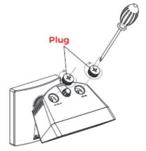
• Replace the threaded Plug with the O-ring on the side of the Flood Light.
