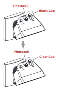
• To use the built-in Photocell function: Remove the black cap and replace it with the clear cap.
