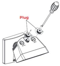
• Remove threaded Plugs from the top of the fixture to access the selection switches.
