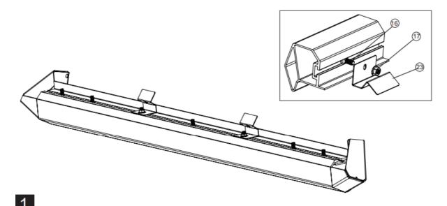
Using Flange Nuts (17), assemble Brackets 2x (25) & 1x (26) onto the rail (4), using the carriage bolts (16) left from previous step. Next, install Flange Bolt (14) and Flange Nut (17) onto bracket tab. Driver side shown. Dimensions shown are for reference.
