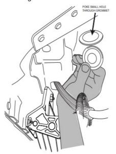
Connect harness to motor. Secure harness with tie wraps (19).
