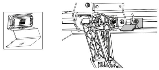
Using supplied butt connectors (22), connect the lamp wires. Red to Red, Black to Black. Once Crimped use heat gun to shrink tube. Close and wrap conduit with electrical tape. Secure all loose wires with cable ties. Pull lamp wires upward to avoid any wire snagging.
