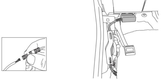
OBD II install: Use Supplied Posi-Lock™ connectors to attach the Plug and Play Module to the Harness. Attach
