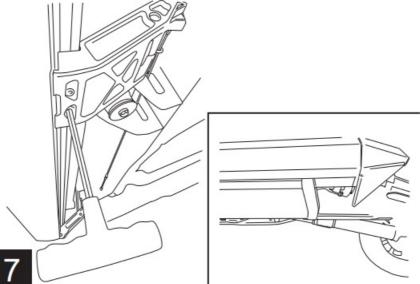
Using a 13mm socket Torque linkage bolts 4x (9) from step 5 to 16 ft-lbs Next use a 10mm socket, torque linkage spacer bolt 2x (13) from step 6 to 8 ft-lbs. Once linkages are tight cycle board to verify steps deploy under own weight.
