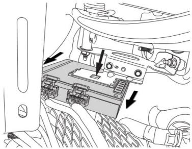
Locate the following wires (black connector) and connect the blue and white wires of the Powerstep Connection Module with supplied Posi-Tap<sup>TM</sup> (8) to the following wire colors listed below.
