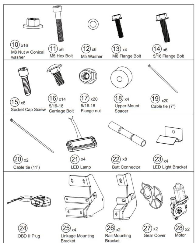
Insert 7 Carriage bolts (16) into slot on rail (4). Insert from either end of rail. Add 2 Light Brackets (23) on the 3rd and 5th bolt. Insert Flange nut (17) onto bracket tab to attach light brackets into position shown. Leave loose to allow for adjustment.
