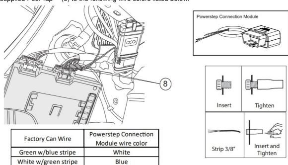
Use supplied Posi-Lock<sup>™</sup> (7) to attach the 2 purple wires of the OBD harness to the main harness. Attach matching colors on the harness to the wires on the module. Lastly reinstall Factory OBD port removed in step 20. Plug in module to OBD port on the vehicle. Reinstall sill plate removed from step 15.
