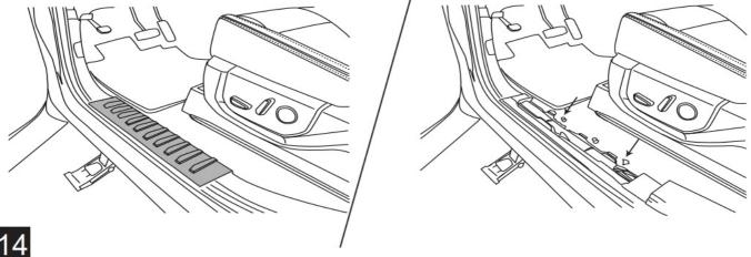
Remove grommet in floor panel above front linkage on driver side. Poke small hole into grommet and thread the two trigger wires through and up into the cabin of vehicle. Seal grommet with silicone sealer.
