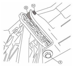
10. Slide mounting T-nut into position, Center board in rail pocket. Tighten fasteners to 10 ft-lbs.
