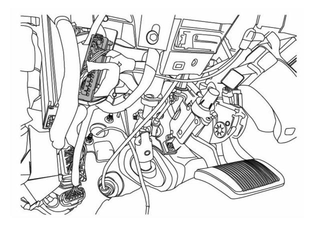
• Plug 2 pin plug into the Green Connector Block. Use supplied Posi-Lock™ (8) connectors to attach the Plug and Play module to the Harness. Attach Matching colors on the harness to the wires on the module. Plug in OBD II module (30) to the OBD II port on the vehicle.
