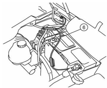
18. Locate large rubber wire boot on driver side firewall as shown below. Slice small opening as shown below to
