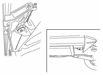
11. Using a 13mm socket Torque linkage bolts 4x (9) from step 3 to 16 ft-lbs. Next use a 10mm socket, torque linkage spacer bolt 2x (13) from step 6 to 8 ft-lbs. Once linkages are tight cycle board to verify steps deploy under own weight.
