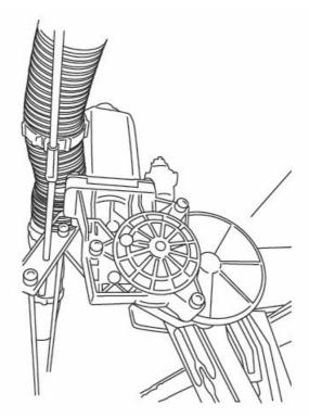
14. Prepare large tie-wraps for mounting Power Step Controller. Loosely loop tie-wraps around large bundle of wires behind battery in engine compartment.
