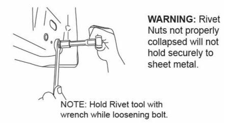
5. Once rivet nuts are in place use a screwdriver to push back tab in hole to avoid interference with linkage mount.
