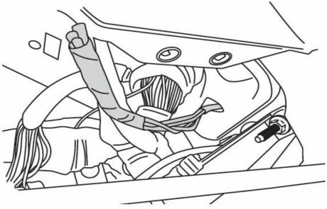
20. Route the two Wire Harness legs down over the wheel wells toward Motor Linkages, long leg across to the passenger side. Secure harness with tie wraps (24).
