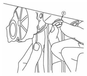
9. Install provided spacer (22) and M6 bolt (13) into upper mount as shown on both the Drive and Idler linkages. Do not tighten.
