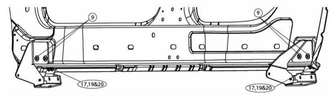
7. Insert and position 6 Carriage bolts (16) into slot on rail (4). Insert from either end of rail. Using Flange Nuts (10) provided assemble rail to Brackets using the 2 outer bolts on each side. Next install Flange Bolt (14) and Flange Nut (10) onto bracket tab. Torque flange nuts to 16ft-lbs. Install Light Bracket (29) using Flange Nut (10), leave loose to allow for adjustment. Driver side shown. Dimensions shown are for reference.
