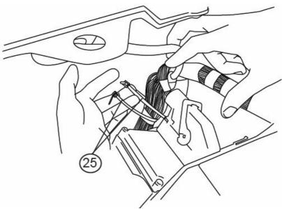
15. Insert controller into tie-wrap loops and cinch down securely. The tie-wraps should cinch down into channels on controller surface.
