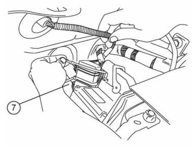
16. Remove fuse from Power Step Wire Harness.
