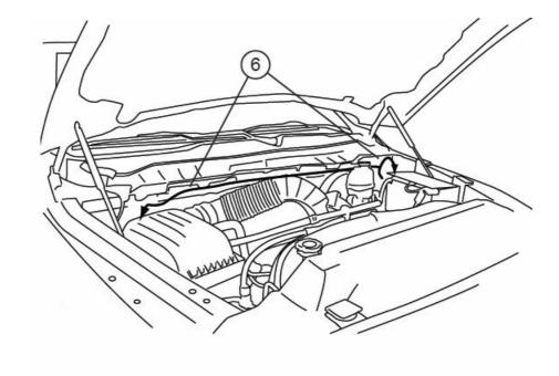
21. Connect harness (6) to motor (32). Secure harness with tie wraps (24) .
