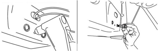
4. With Rivet Nut Tool held in place with 19mm wrench, tighten Hex Bolt until Rivet Nut deforms and secures itself
