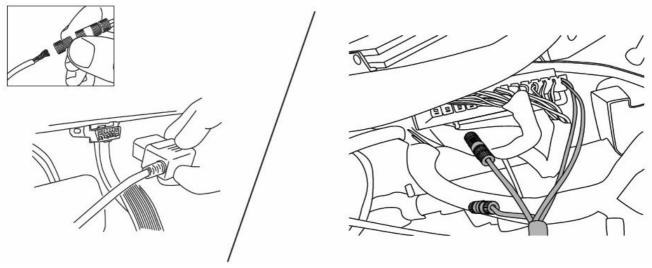
• Secure harness with supplied tie wraps. Make sure wires are away from E-brake mechanism and brake pedal assembly.
