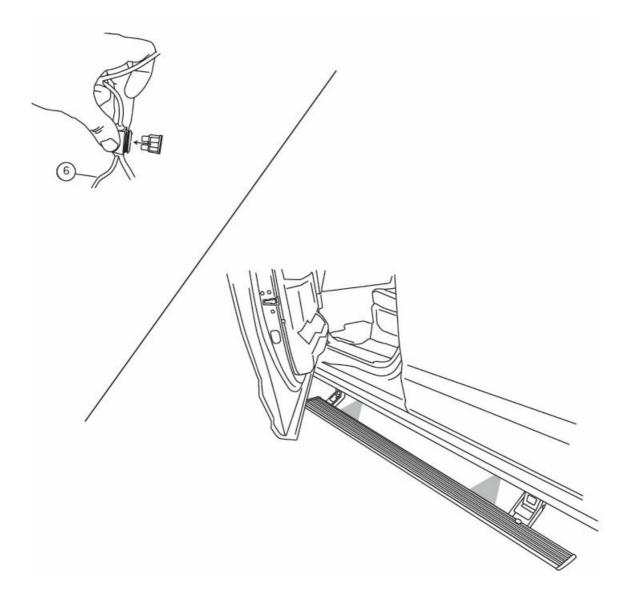
Check that all doors activate the PowerStep and the LED lights work when doors open and close.
