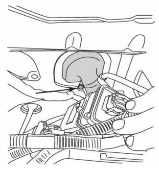
19. Tape leading end of wires together and push through rubber boot to cabin side of the firewall. Silicon lubricant may be used for ease of passage. The trigger wires will come out just above and to the left of the brake pedal.
