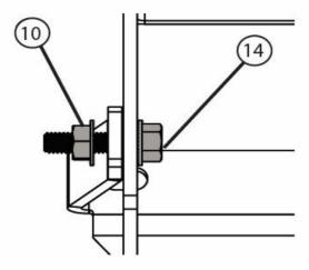
13. Attach motor to linkage. Using a 4mm hex, torque to 36 in-Lbs.
