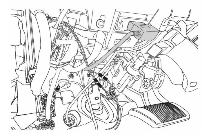
**OBD II install:** Use Supplied Posi-Lock connectors to attach the Plug and Play Module to the Harness. Attach matching colors on the harness to the wires on the module. Plug in module to OBD II port on the vehicle. Secure harness with supplied tie wraps.
