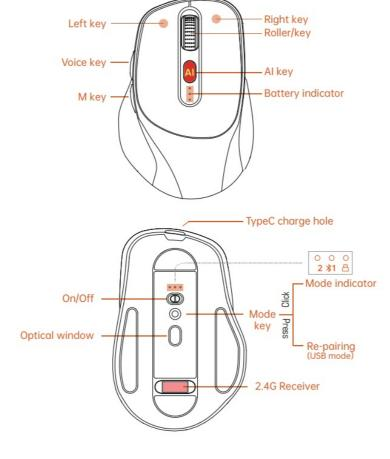
This product supports two connection modes: USB (2.4G) and Bluetooth (BT3.0 or BT5.0) for wireless connection to computers. After turning on the mouse power, pressing the mode switch button can switch the connection mode.
