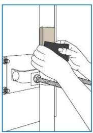
5. Wrap the tape with  $\frac{1}{2}$ " overlap and use minimal tension.
