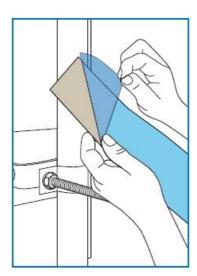
2. Adhere one end of the absorber stripe to the pole and wrap the absorber around the surface.
