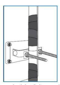
8. Apply "Do Not Remove" label around the previously installed tapes and place additional labels as desired.
