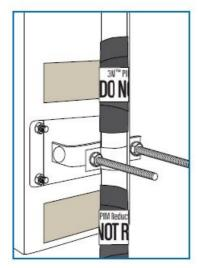
10. Apply 3M™ Scotch® Tape 130C with no stretch, apply 1″ beyond absorber. Proceed from bottom to top.
