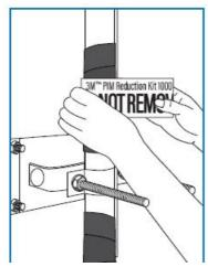
9. Remove absorber liner and apply above and below bracket attachment location, allow 2" gap.
