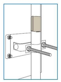
4. Apply 3M™ Scotch® Linerless Rubber Splicing Tape 130C 1″ beyond absorber. Wrap from bottom to top.
