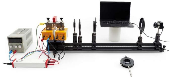
Fig. 1: Experimental setup for the normal Zeeman effect in a longitudinal configuration
