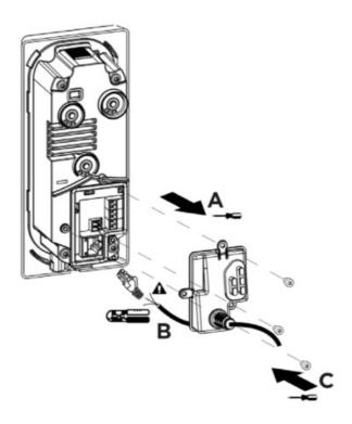
Insert the metal device body into the walled-in box and fit it on the bottom using a Torx head screw.
