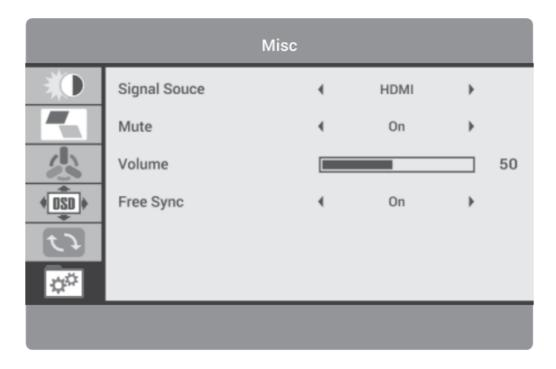
$\mbox{{\bf HDMI}}-\mbox{{\bf Sets}}$  the HDMI port as the monitor video source.
