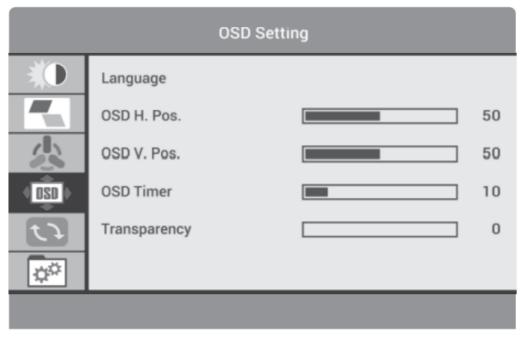
**OSD H.POS.** -This setting allows you to adjust horizontal position of the on-screen menu.
