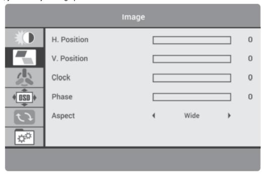
**H.POSITION** – This setting adjusts horizontal position of the image.
