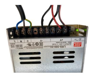
• Connect the power supply pins of the power supply to the GigaSync paying attention to the polarity adopted. (Ref. Q&A 1 Fig.2)
