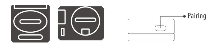
6 button mode <=> 3 button mode switching can be achieved by pressing mode button on the controller for 3 seconds. LED on the receiver will blink twice to indicate the change
