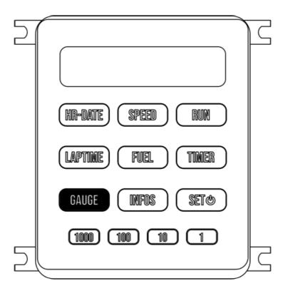
**INFORMATION.** Successively press to display outdoor temperature (if equipped), accelerometer, current heading, and altimeter.
