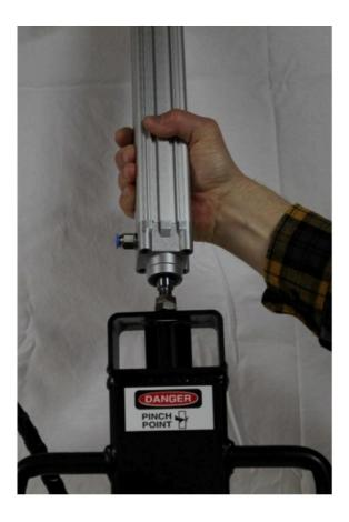
With a lock washer on each screw, hand-thread all four of into the air cylinder.
