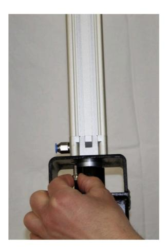
Using the supplied Hex Wrench tighten all four screws. These screws can work lose over time, so they must be periodically checked. A thread-locking adhesive can be used on these as well.
