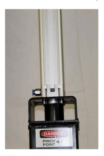
Finally connect the two airlines, and thread in the exhaust muffler and your assembly is complete.
