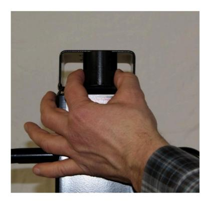
Place the air cylinder into position making sure the fittings are facing towards the push button valve of the post driver
