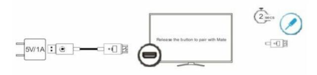
2 Connect the transmitter to the computer, When the TV/monitor shows "Ready to pair", press the button of the transmitter for 5 seconds and wait until the indicator is off, Pairing is complete.
