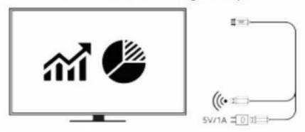
Plug the HDMI port(②) of the transmitter into a laptop or other device with HD video output function, and use our included USB-C to USB-A cable to connect a power supply and the PD3.0 port(③) to power the transmitter. After the indicator light enters the fast flash state, wait for 10 seconds to complete casting.
