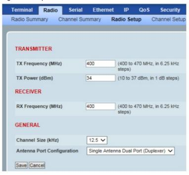
You can now configure the remaining Data-Driven Protected Station and network parameters and settings. For more information, please refer to the Aprisa SR+ User Manual available from the 4RF website <a href="https://www.4rf.com/secure">https://www.4rf.com/secure</a> (login required).
