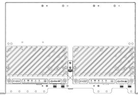
The Aprisa SR+ Data-Driven Protected Station has an earth connection point on the left top of each radio. Use the supplied M4 screw to earth the enclosure to protect earth.
