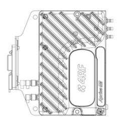
The Aprisa LTE has an earth connection point on the top left of the enclosure. Use the supplied M4 screw to earth the enclosure to protect the earth.
