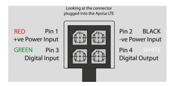
The Molex Micro-Fit 3.0 4 pin connector clips into the Aprisa LTE socket. It also has a locking plate and screw (supplied with the Aprisa LTE) that enables the connector to be secured to the Aprisa LTE with a screw.
