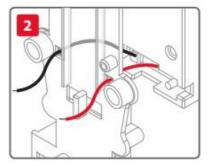
3. Lower the battery case onto the body plate so that the pegs in the battery case slot into the holes in the body plate. Be careful not to trap the wires between the battery case and the body plate. Fix the battery case in place with two screws through its base. Do not put a battery in the case yet.
