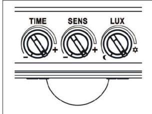
→ - Approx. 8m Max ⊕ - 10 seconds to 7min Ф - 3 Lux - 2000Lux
