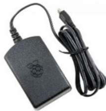
5V DC Supply Suitable for the BeagleBone Black (using DC Jack), recommended 2A @5V
