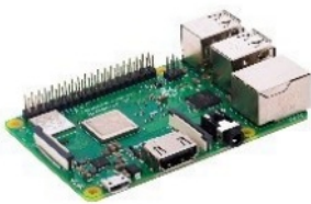
Raspberry Pi board Compatible with Raspberry Pi A+, B+, Pi2, Pi3, Pi3 B+, Pi4, Pi Zero and Pi Zero W
