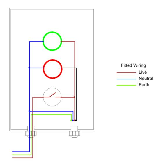
The control panel is supplied with wiring installed in the drawing shown above. The level sensor needs to be fitted as shown in the next diagram.
