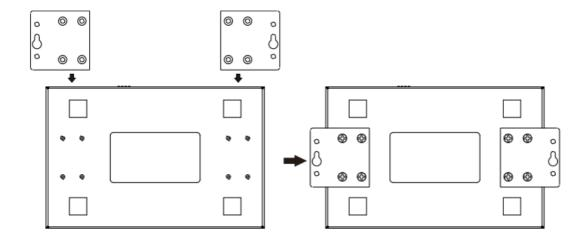
**Step 2** On the wall of device mounting, place the device on the wall for reference or refer to the mounting dimension to mark two screw positions.
