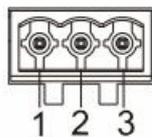
This device provides 1 DC power supply which is 3-pin 5.08mm pitch terminal blocks, the power supply supports non-polarity. Voltage range: 12~48VDC. The pin definitions of the terminals are shown as follows:
