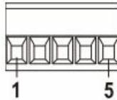
This device provides 1 RS-485/422 serial port, support RS-485 or RS-422, and Interface adopts 5-pin 5.08mm pitch terminal blocks.
