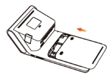
**WARNING** This device uses a custom battery. Do not replace it with any other types of batteries. CAUTION: Using an incorrect battery may cause an explosion which can lead to severe injury or death.
