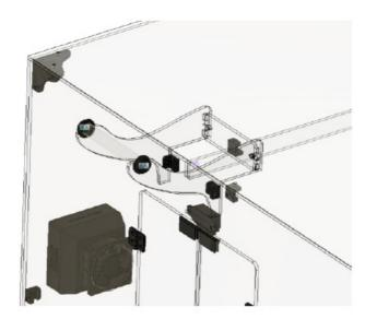
The filament feeds into the extruder through the gaps in the side doors. Position the enclosure from front to back so that the slit lines up with the extruder's filament input hole.
