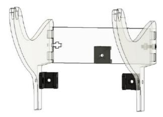
Although the end caps should fit snugly, you should glue them on with superglue just to be safe.
