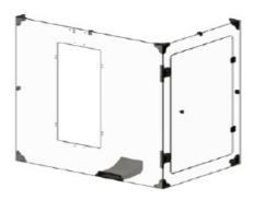
The CR-10 Max design adds a side door for easy access to the extruder. The latch mounts are smaller than the front, although the magnetic latch attaches in the same way with wood screws. The parts for the side door will be in a separate packet.
