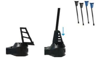
These legs are a tight fit and require considerable force to remove. Because of this, be careful not to place your fingers in the path of the leg as you remove it. This can expose your hand to the sharp edge of the leg when it pulls free of the arm. We recommend using your thumbs to push the leg out while ensuring that your other fingers are away from the end of the arm.
