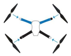
Each propeller has locking and unlocking direction symbols. To attach, spin the propeller in the direction of the locking symbol. The propellers will automatically tighten onto the motors when you arm IRIS before takeoff.
