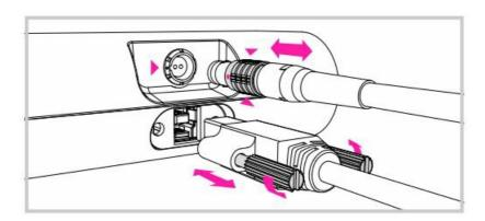
Plug the device cable into the port of the scanner, make sure the red dot is lined up with the groove on the port; To unplug the cable, move backwards the bushing (as marked with the red triangles) and pull out the cable directly.
