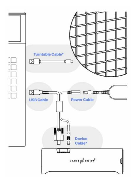
Plug one side of the data transmission cable (as it's showing Device Cable) into the scanner, another into the computer USB port and power adapter; The turntable cable is for powering up the turntable.
