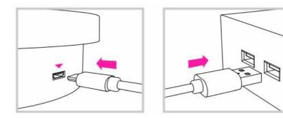
The turntable can be powered up by connecting it to the computer or the power adapter with the turntable cable.
