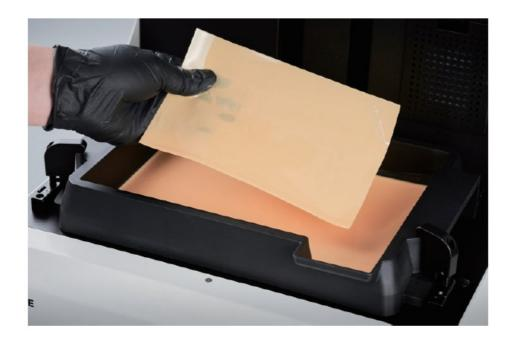
Cover the resin tank with a lid if the resin material needs to be stored within the tank temporarily. Please take resin material out of the tank if it will be not consumed in 3 days, make sure to get it filtered before storing it in a light-proof container. It was not recommended to mix it with the original one directly.
