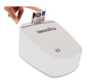
1. Insert the identity card/driving license fully, so that it locks in place with the latches on both sides. Let the card remain still during the scanning process.
