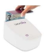
Be extra careful with passports that have a thin data page to ensure it is not damaged. Insert the passport until it does not insert any further.
