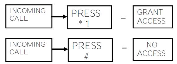
On the mobile Phone, press \* followed by 1 or \* followed by 2 (to trigger Output 1 or 2) to grant access (this will pulse the relay).
