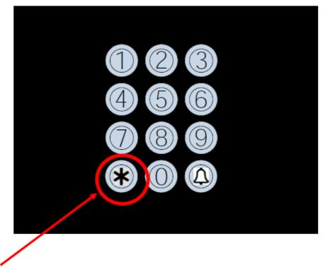
Should you make a mistake when entering a code and need to start again, then simply press the Star button ( $^*$ ) as highlighted above to start again.
