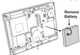
**WARNING:** Avoid the use of sharp tools or aggressive prying, because this could damage the battery or panel.
