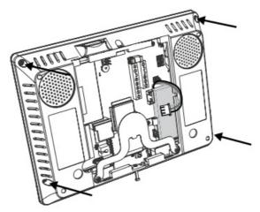
5. CONNECT POWER. Connect the barrel connector, or if it is hard wired, insert wires and tighten the screws to hold them in place.
