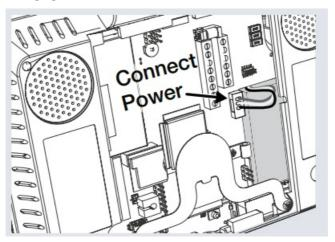
7. MOUNT THE EDGE PANEL: Align the EDGE panel on the backplate, then carefully snap it back into place.
