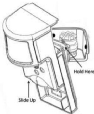
Figure 4. Removing Sensor for Battery Replacement
