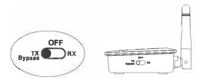
Switch to Trcnsmitter+Bypass mode/ Power off/ Receiver Mode
